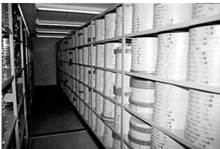
Figure 2.2. Cold storage vault, set at 40°F and 30% RH, with films shelved horizontally.
