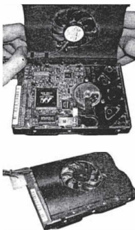
3.16-rasm. Vinchesterga sovitish qurilmasini o'rnatish.
