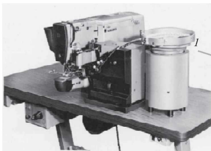
73-rasm. LK-981-555/BR-2 tugma qadash yarimavtomatining tashqi ko'rinishi.
