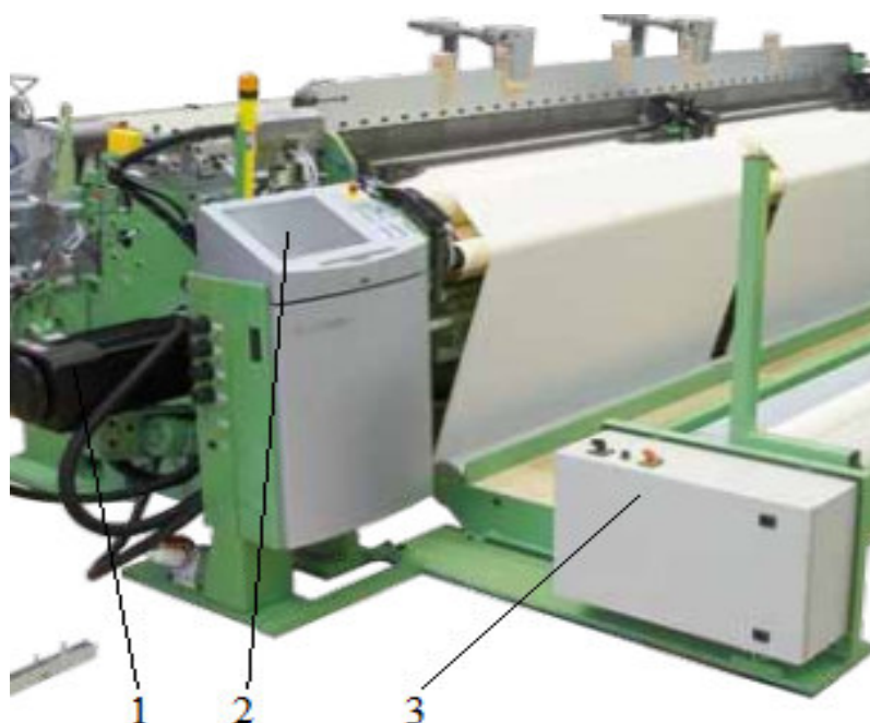
9.8-rasm. DORNIER to'quv dastgohi 1- DORNIER SyncroDrive motori, 2-boshqaruv paneli, 3-elektroquti.
