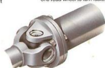
Universal joint The commonest type of universal joint, the Hooke joint, uses a cross-shaped 'spider' across the axis of the drive shaft. The
