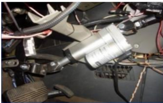
c) Avtomobil tormozining pedali 1.9 rasm. Avtomobil eksperimental tizimini yig'ish
