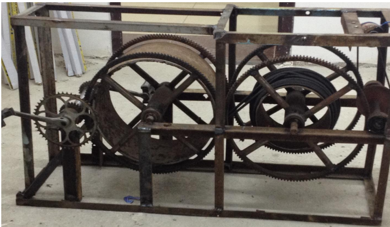
3.2 – rasm. Standart o‘lchamdagi jihozlardan foydalanib tayyorlangan muqobil energiya manbaining tajriba modeli.
