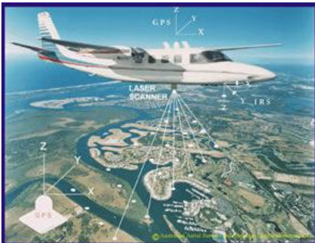
7-rasm. Lazerlokatorining ishlash prinsipi.
