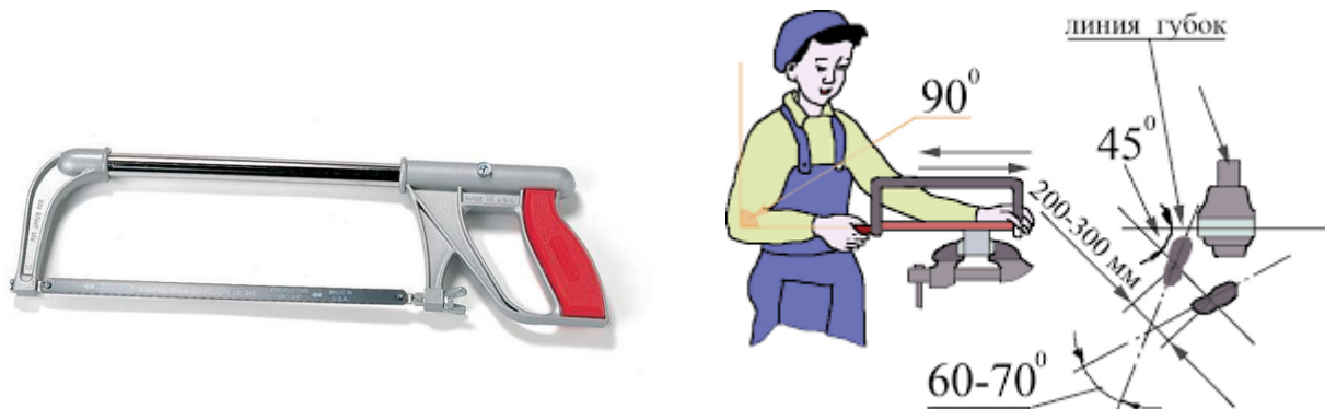
2.5-rasm. Dastaki arra va arralash usli..
