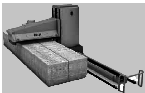
2-rasm. Blendomat BO-A (Truetzschler) avtomatik toy titish mashinasining ishlashi
