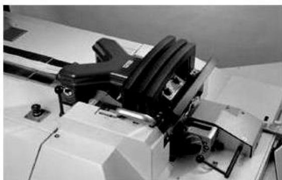
63-rasm. Truchler firmasi tarash mashinasining cho'zish asbobi
