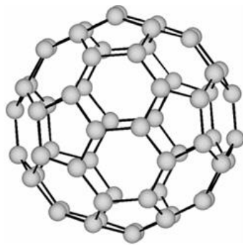
2-rasm.C 60 fullerening sxematik ko'rinishi
