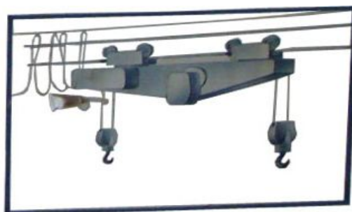
3.3-rasm. Jinlashssexidagi elektrotelfer.
