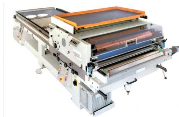
34.4-rasm. Svetoproba tayyorlash uchun tekis ofset bosma sinov bosish dastgohi
