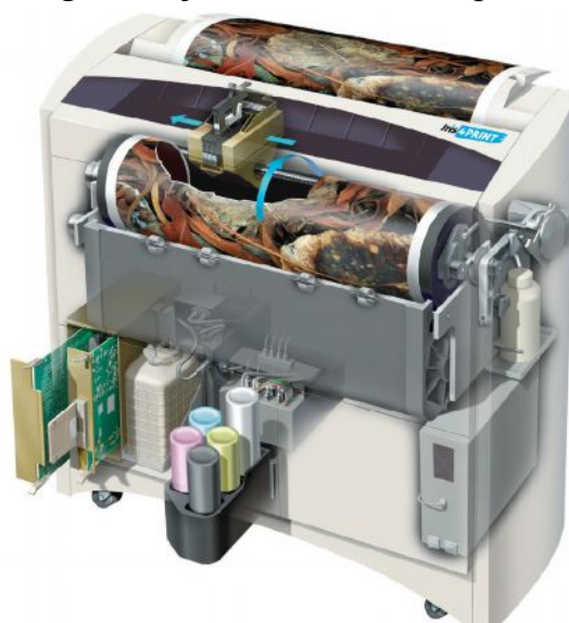
34.5-rasm. Svetoproba tayyorlash uchun purkashli bosma tizimi (Iris 4 Print, Scitex)
