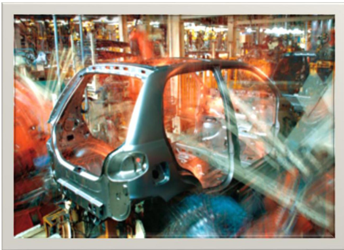
1-rasm: Matiz avtomobili kuzovini payvandlash jarayoni
