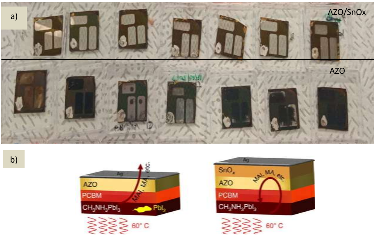
Figure 12: a) Photographs showing the colour change (the corrosion of metal electrode) upon thermal stress under the same high vacuum conditions (10 -4 mbar; 60 °C). MAPbI 3 device with and without SnO x . b) Schematic illustration depicting the suppression of degradation pathways through the incorporation of an ALD-grown internal SnO x barrier.
