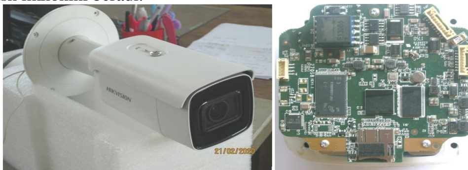
9-rasm. A12A55 videoprotessori asosidagi Hikvision DS-2CD2625FWD-IZS videokuzatuv kamerasi va boshqaruv platasining tashqi ko‘rinishi
