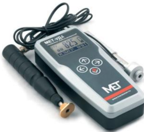
Rasm. MET-UDA –universal qattqlik o'lchagich
