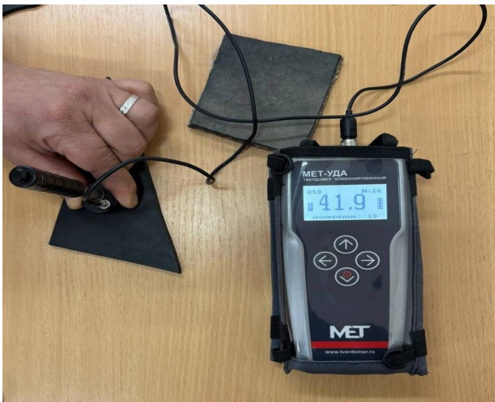
3.3-rasm. Kauchukning qattiqligini o'lchash jarayoni (TCK 10, TSK 1 OCV
