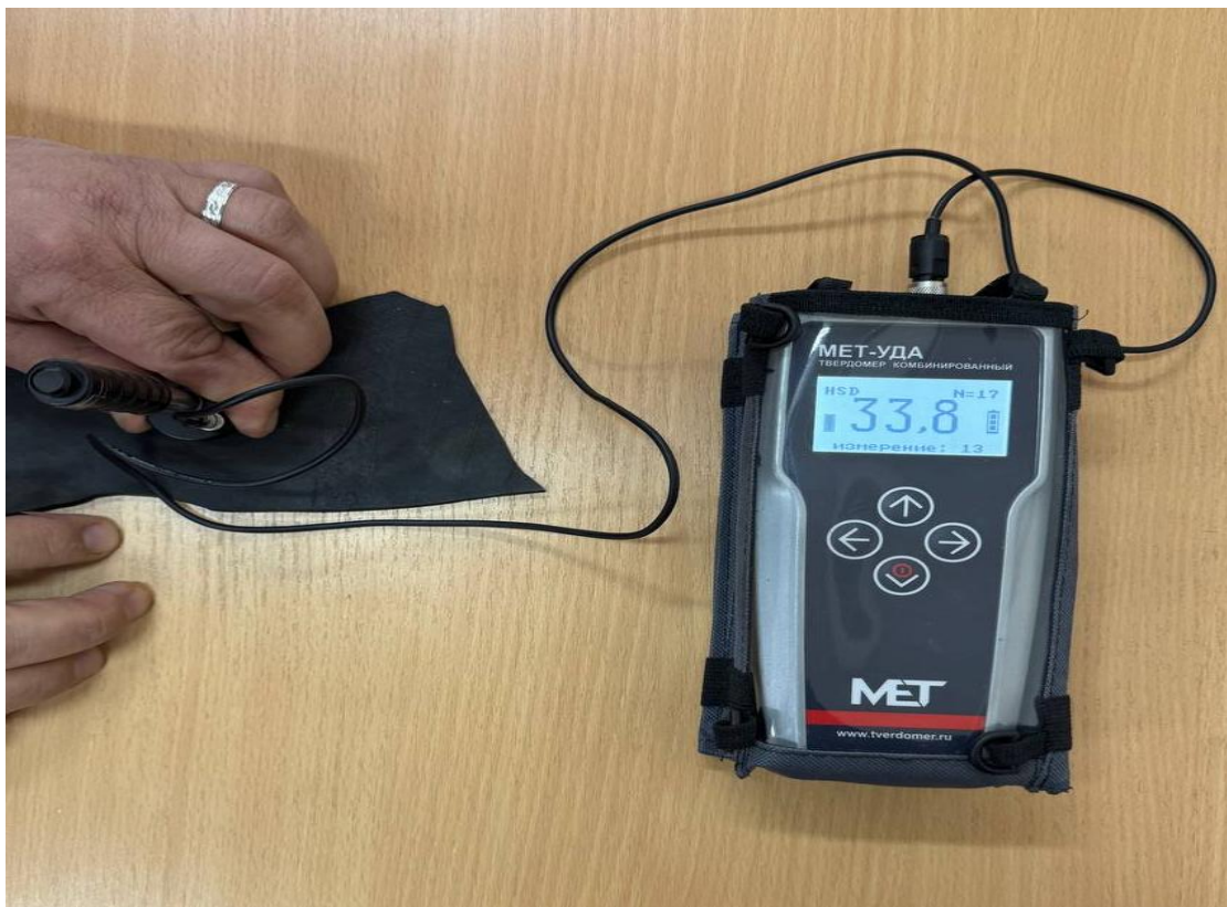
3.2-rasm. Rezinaning qattqligini o'lchash jarayoni Rezina markadagi material (TMKSh)
