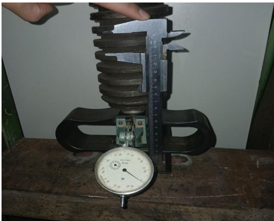
3.11-rasm. Lenta materialining bikrligini o'lchash jarayoni (material qalinligi 3,5 mm)
