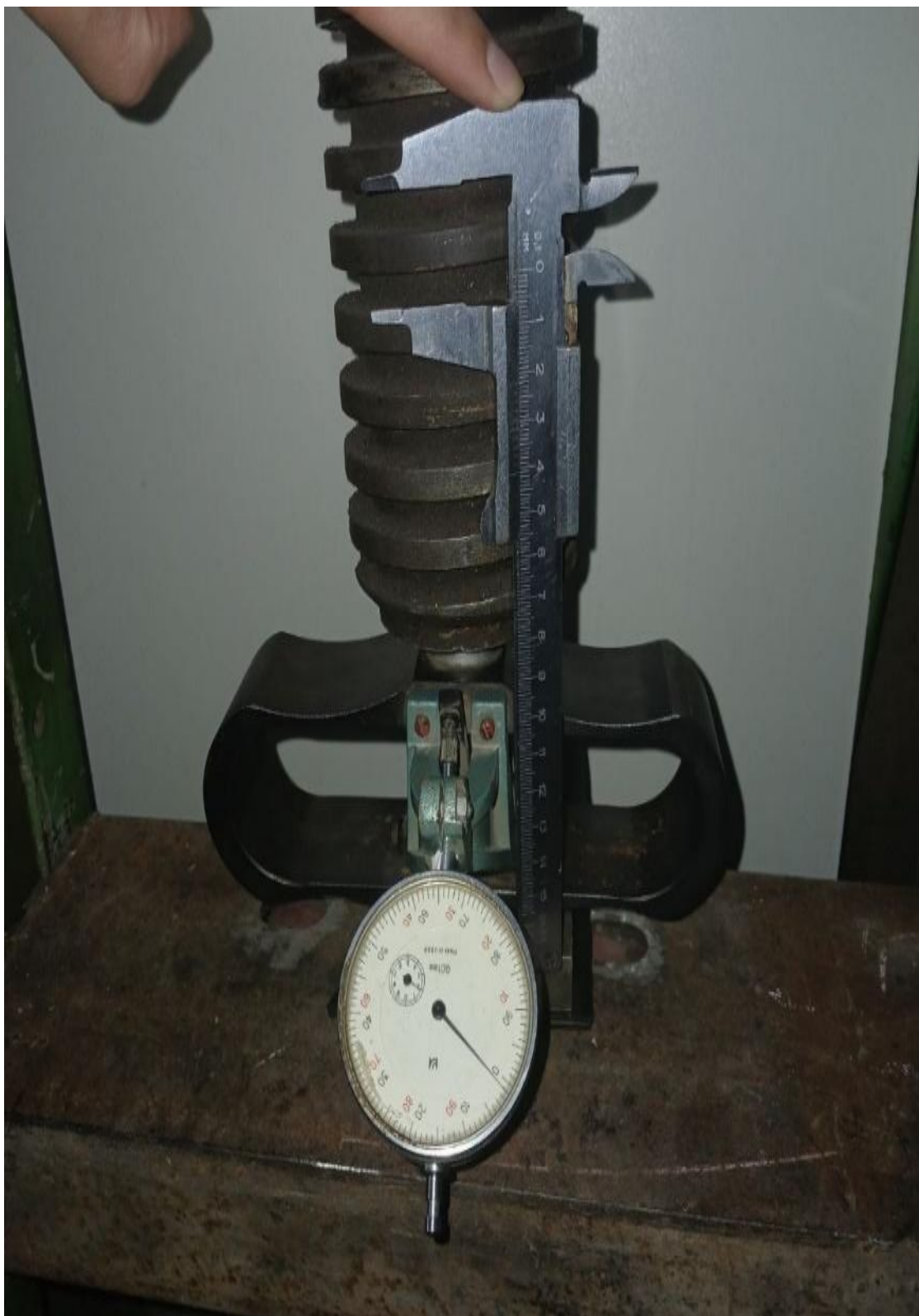
3.10-rasm. Lenta materialining bikrligini o‘lchash jarayoni (material qalinligi 3,0 mm)
