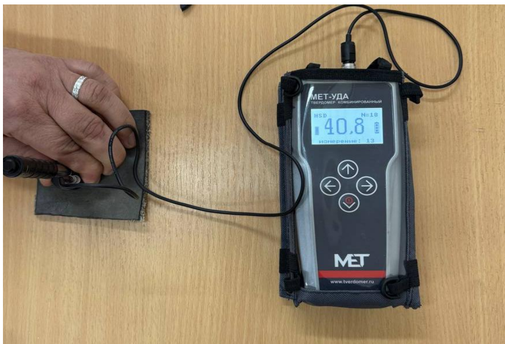
3.4-rasm. Konveyer lentasining qattiqligini o'lchash jarayoni (2T1-800-6-TK-100-8-2-T-1-NB GOST 20-85)
