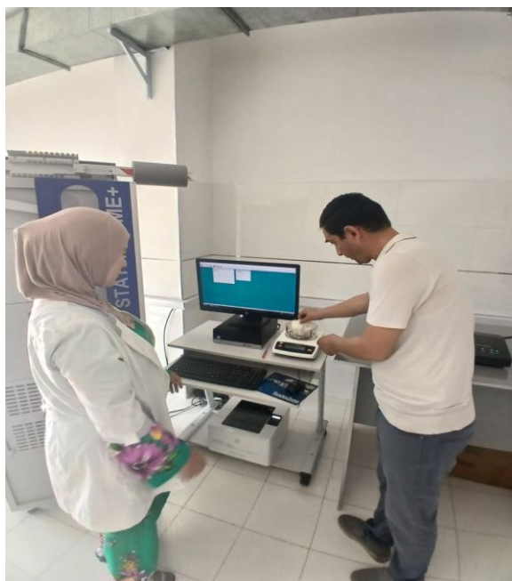
9-rasm. Sinov uchun namunani massasini tortish jarayoni
