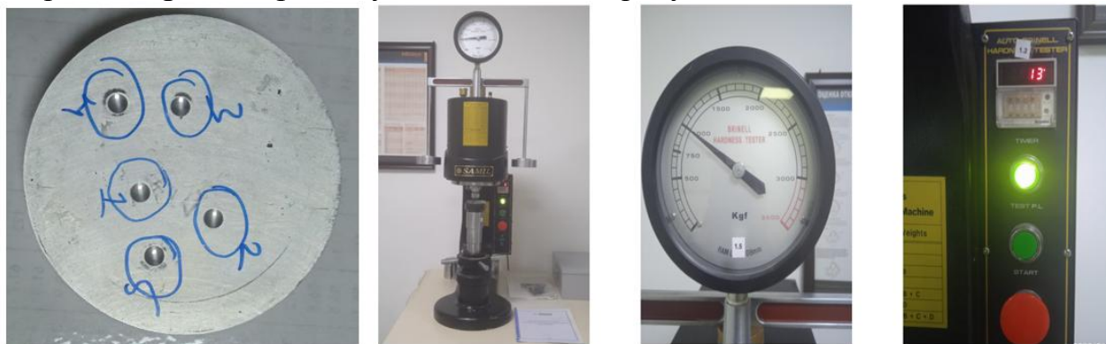
5-rasm. Tadqiqot namunalarini Brinell usulida qattqligini aniqlash jarayoni
