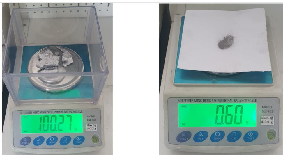
2-rasm. Shixta miqdoriga bog‘liq holda Ni zarralarini kiritish.
