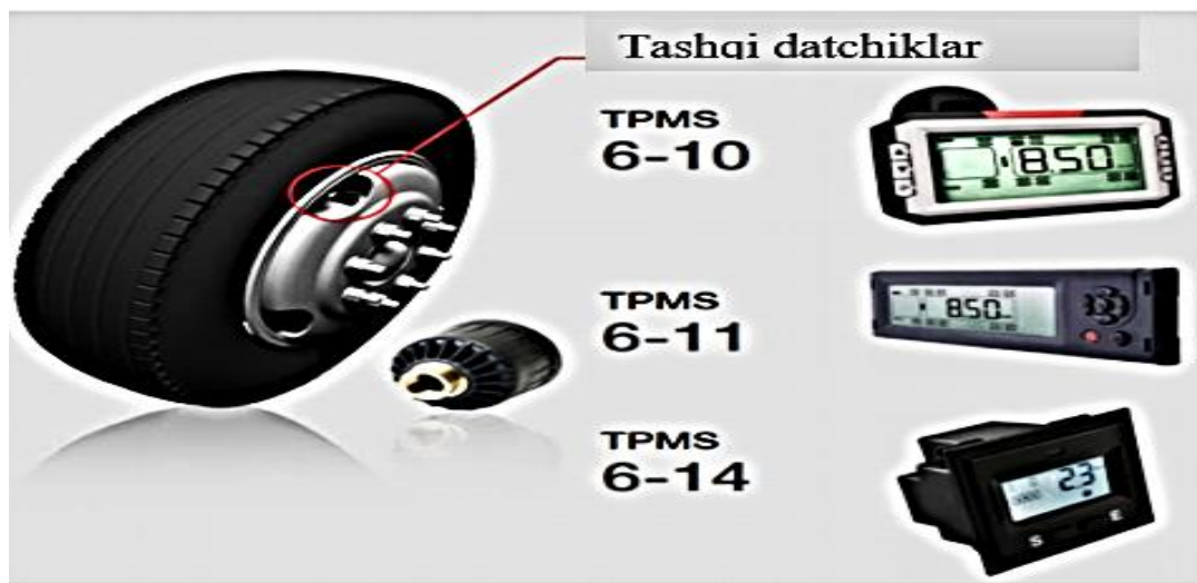
7-rasm-Tashqi sensorlarga asoslangan monitoring tizimi
