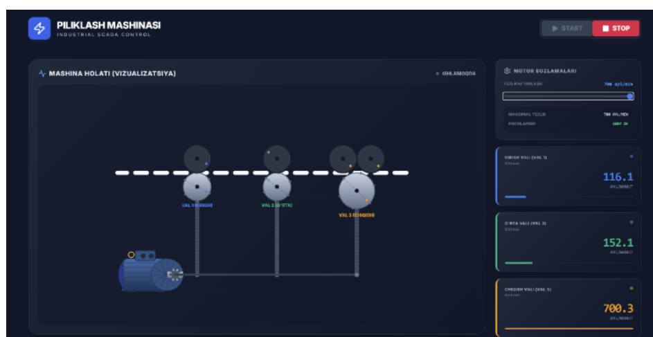
8-rasm. Piltalash mashinasi SCADA bosh ekrani (HMI interfeysi)
