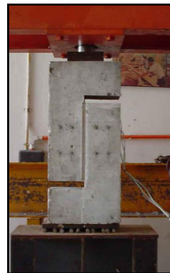
4.11-rasm. Maxsus namunani yuk ostiga o'rnatish
