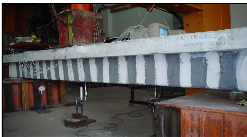
4.34-rasm. Tavr shaklli to'sinni yig'iq yuk ostida egilishga sinash
