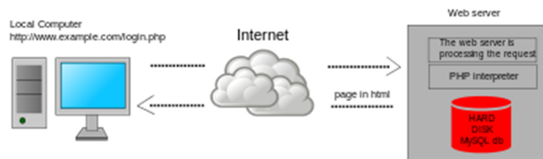
Figure.1. Dynamic web page: example of server-side scripting (PHP and MySQL)
