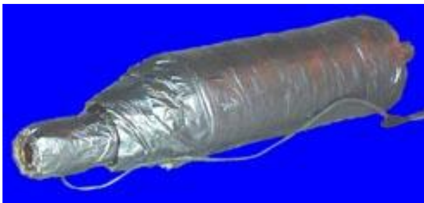
17-rasm. Karl Velsning ozon aralashmasini tayyorlovchi qurilmasi
