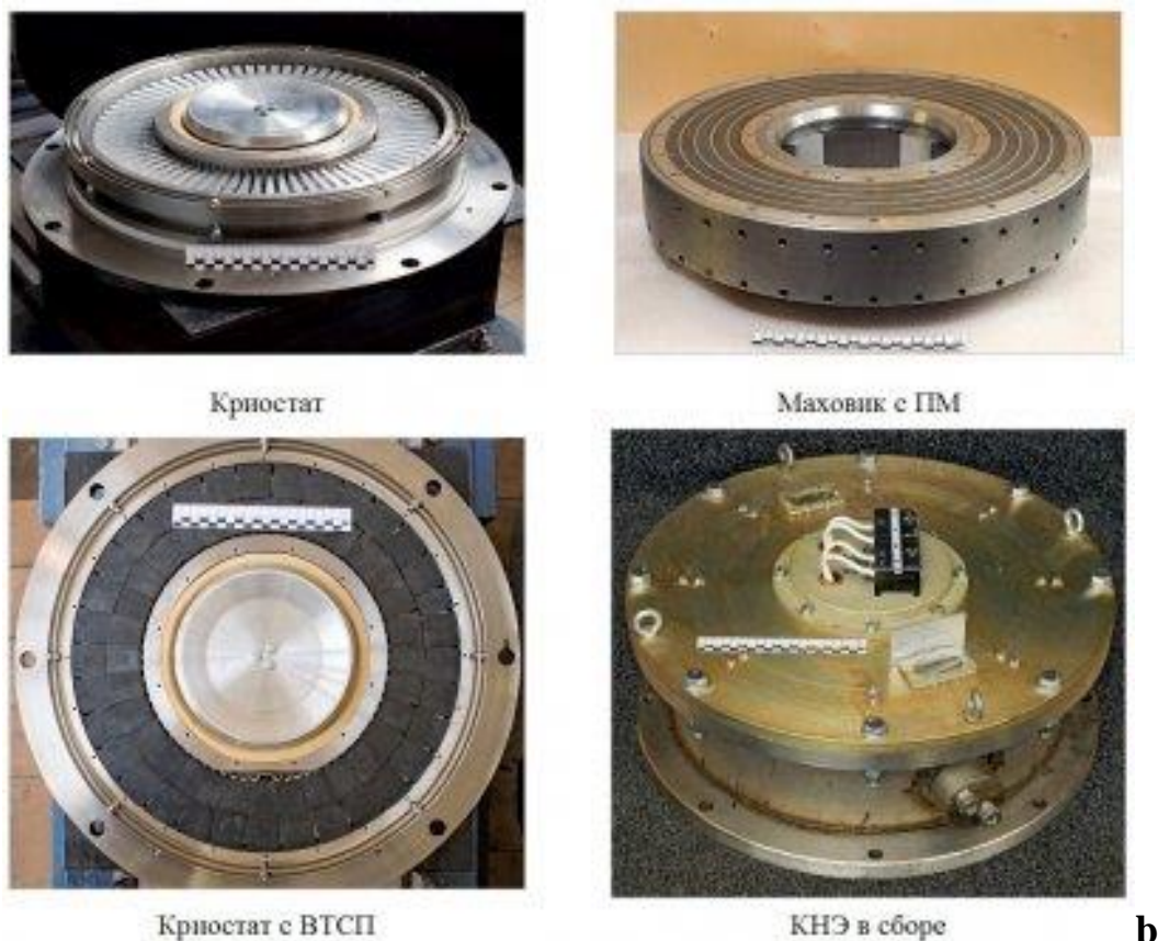
14- rasm. “Beacon Power” energiya to‘plagichining asosiy uzellari
