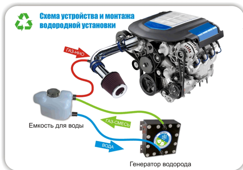
16- rasm. Suv gazi generatorining IYODga ulanishi
