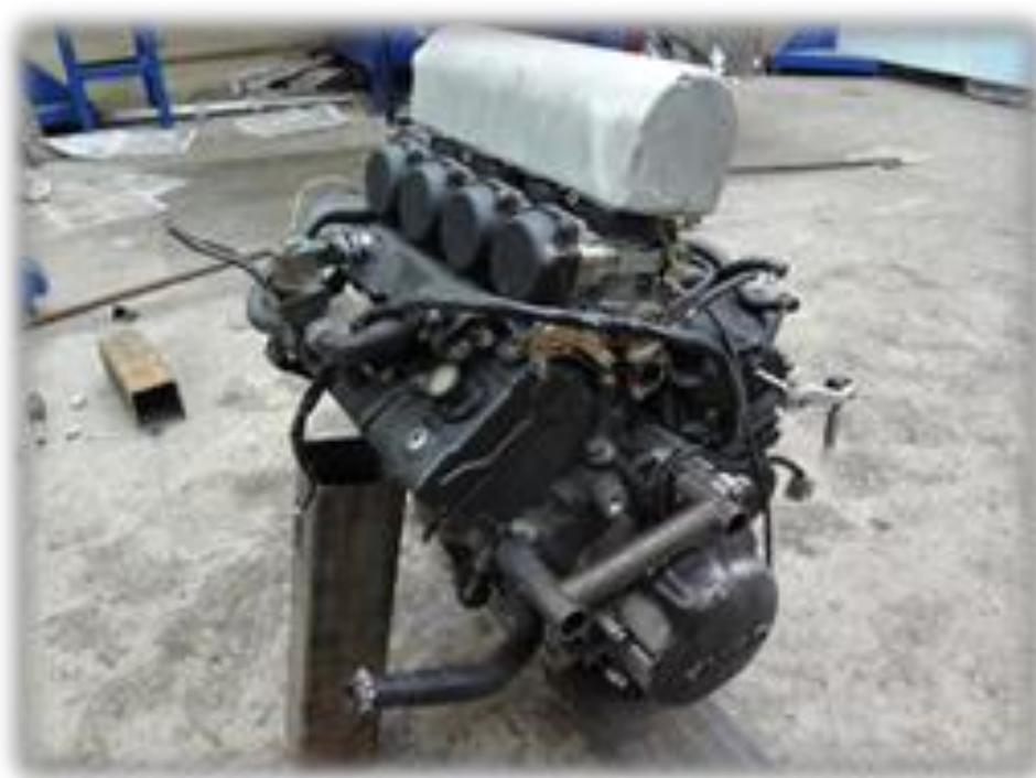
3-rasm. Formula bolidining dvigateli
