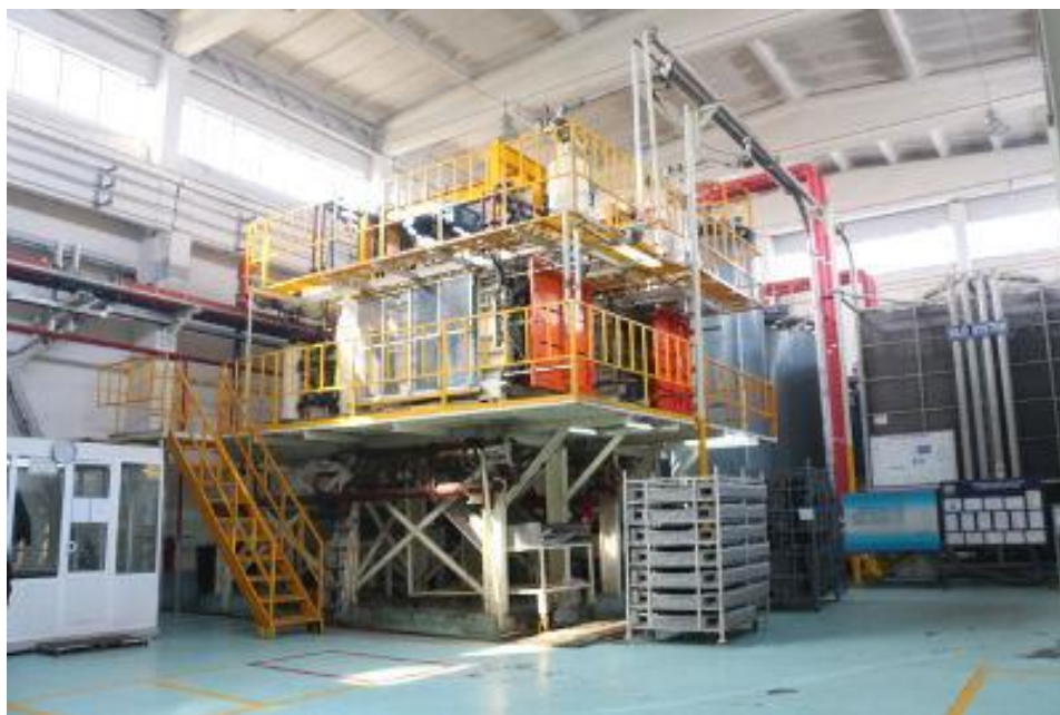
1.3.3 -rasm. Kengayuvchi polipropilendan (g30p) quvvatyutkich quyish.
