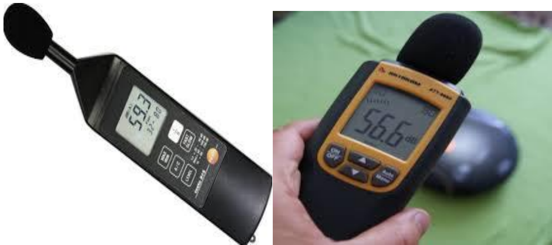
2.4-rasm. Shovqin o'lchagich (shumomer) VZV-003m2, SH-1m30, SH-71 yoki ISHV-1 shovqin o'lchash asbobi.
