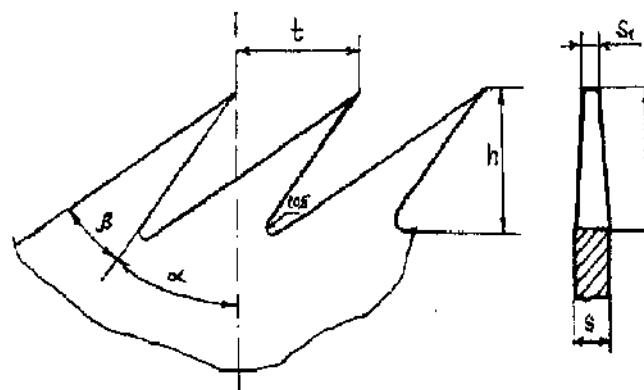
9-rasm. Arra tishmmg geometrik o'lchamlari a =
