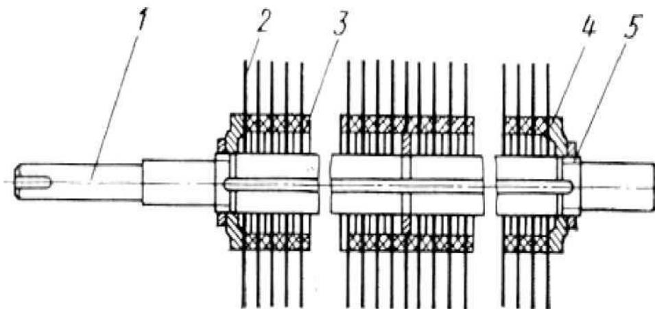
8-rasm. Arrali silindming tuzilishi
