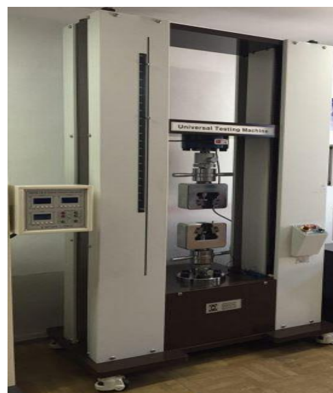
4.4-rasm. Universal test mashinasi
