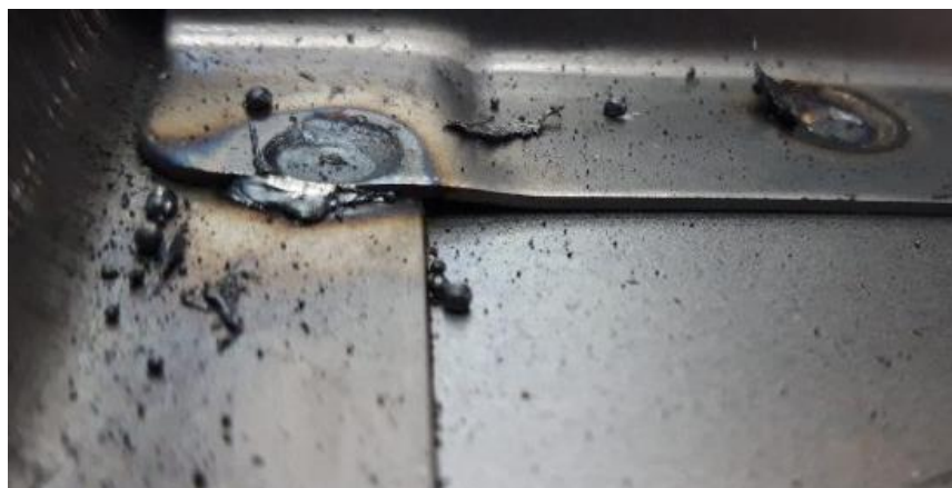
4.2-rasm. Kontakt payvandlash jarayonida ajralib chiqayotgan metall sachramalari oqibatida tayyorlangan panel yuzasining holati.
