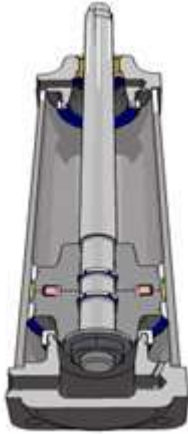
9.14-rasm. 3D-formatdagi pnevmatik porshenli tsilindr qirqimi
