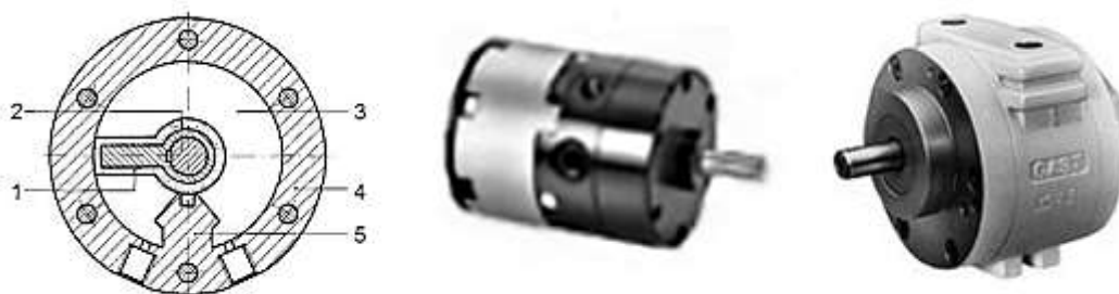
9.25-rasm. Plastinali (shiberli) aylanuvchi pnevmodvigatel.
