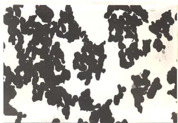
Figure 9. Electron micrographs of tungsten carbide powders on the basis of the standard (s) and "pre recovered" ultrafine (b) h50000.
