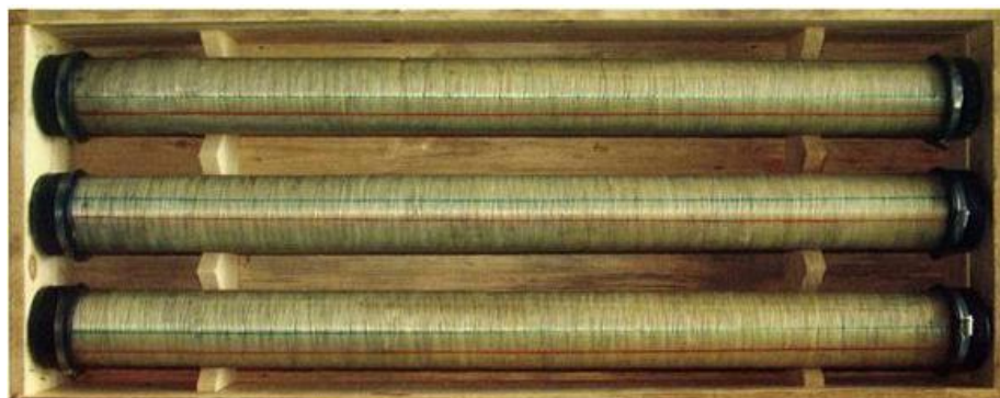
8.2-rasm. Izolyatsiyalovchi kern olish moslamasidan olingan kern
