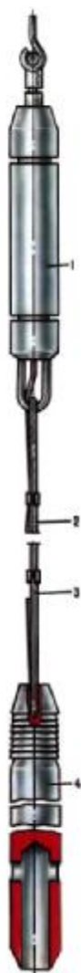
9.6a-rasm. Detonatsiyalovchi shnurli nogermetik Torpeda: 1 - Torpedaning kallagi; 2 - detonatsiyalovchi shnur; 3 - metal tros; 4 - yuk.
