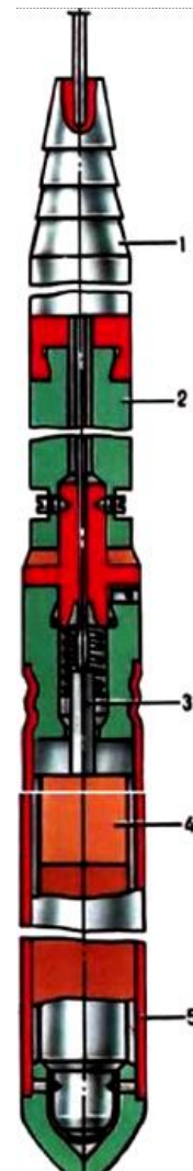
9.6b-rasm. shashkali fugas Torpeda: 1 - Torpedaning kallagi; 2 - yuk; 3 - portlovchi patron; 4 - portlovchi modda shashkasi; 5 - Torpedaning korpusi.
