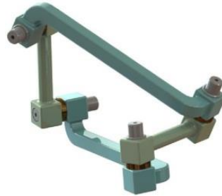
1.21-rasm. To'quv stanogi batanli mexanizmi (1 – qo'zg'almas zveno, 2 – krivoship, 3 – shatun, 4 – batan)
