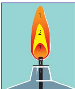
5-rasm. Spirt lampasi alangasining tuzilishi.
