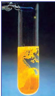
50-rasm. \text{AgNO}_3 va \text{NaJ} dan \text{AgJ} cho‘kmasi hosil bo‘lishi.
