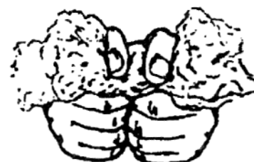
III.11-rasm. Qo'lda shtapel tayyorlash.
