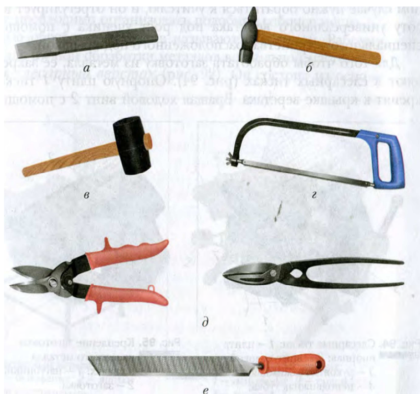
3-súwret. Materiallarǵa qolda islew beriwshi ásbaplar. a- zubila, b- shòkkish, v- toqpaq, g- pishqì, d- qayshì, e- egew.
