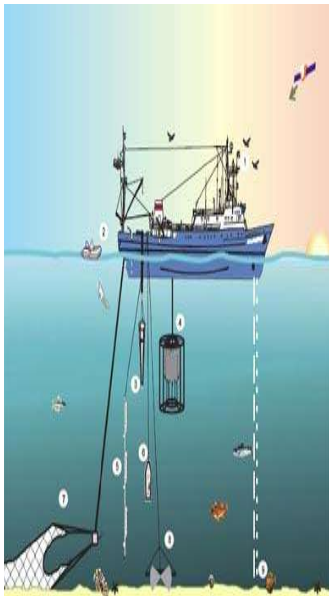
6-rasm. Batometr yordamida ochiq havzasidan suv namunasini olish
