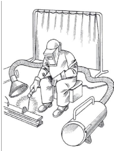
Figure 45. Arc welding – workplace earthed, welder wearing personal protective equipment, workplace screened
