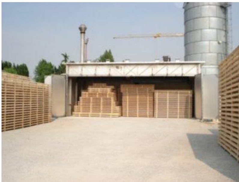
26-rasm. Yog`ochni quritish kamerasi
