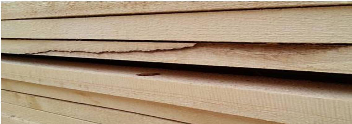
19-rasm. Bo`yiga yorilgan yog`och
