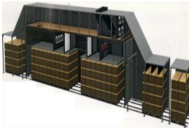
28 –rasm. Standart quritish rejimiga asoslangan quritish kamerasi
