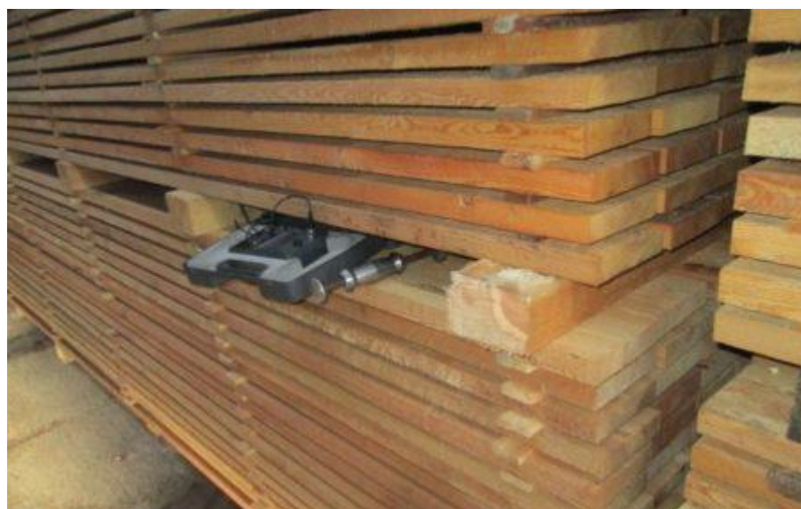
27-rasm. Yog'ochni quritishda ularni taxtlash
