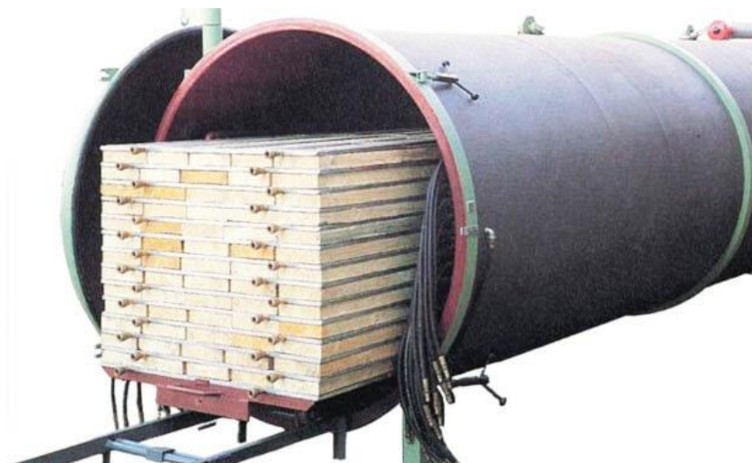
27-rasm. Yog'ochlarni vakkumli quritish moslamasi
