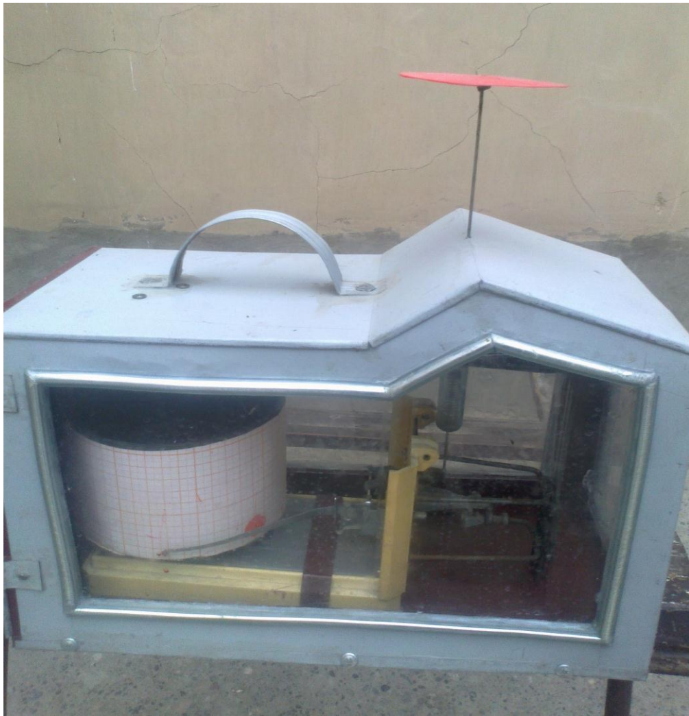
19- rasm. Yog`in jadalligini o`lchash asbobi
