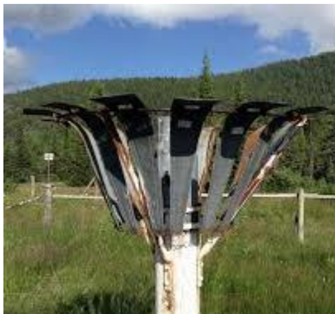
1 - rasm. Tretyakov yog`in o`lchagichining tashqi ko`rinishi
