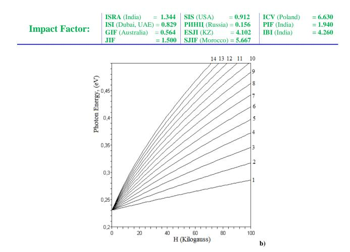
Fig. 5. Changing the maximum energy of the absorbed photon from the strong magnetic field for InSb. a) Experimental data [13], b) calculation of by the formula (11).
