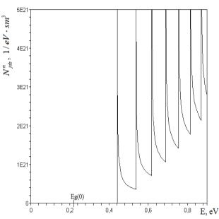
Fig.1. The dependence of oscillations JDOS on the energy absorbed photon in InSb with the nonparabolic dispersion law, calculated using the formula (8). Here, B=5 T.
