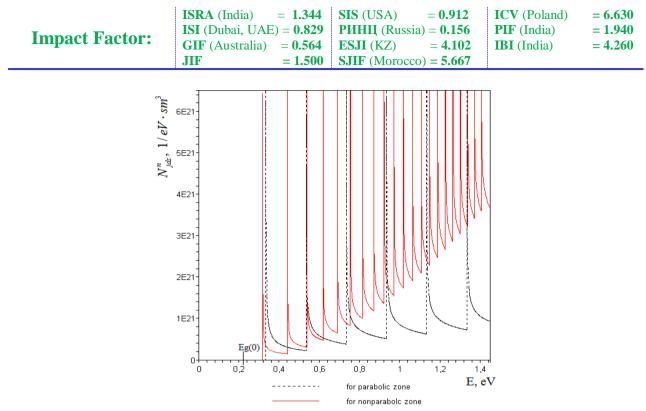
Fig.2. Oscillations JDOS in a strong magnetic field(B=2T.) at the parabolic and non-parabolic dispersion law
