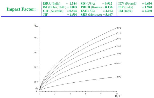
Fig.4. The influence of magnetic field on the maximum frequency of the absorbed light in nonparabolic dispersion law, by the formula (11).
