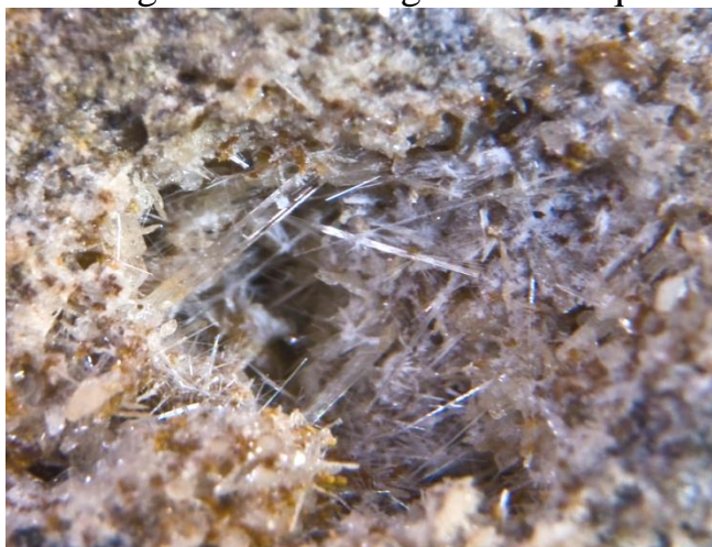
Vollastonitning mikroignasimon tuzilishi (1700 marta kattalashtirib olingan).
