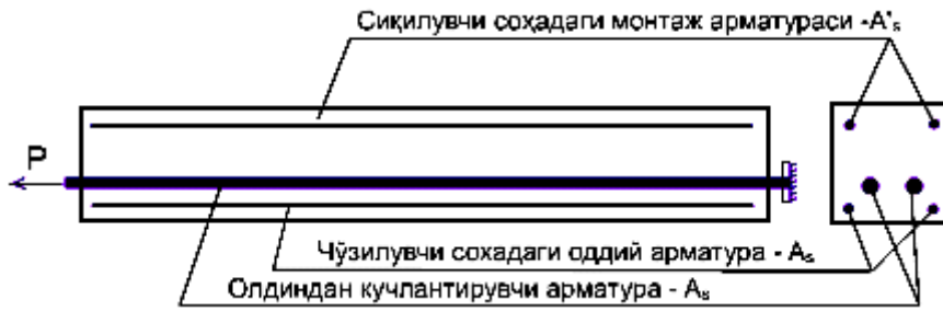
Namunaning bo'ylama armaturalari
