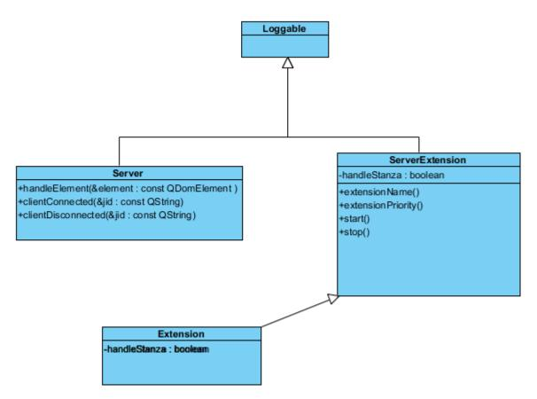
Figure 2.3. Application manager structure in server
