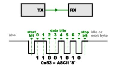
Figure 1.3. Serial port interface bits order
