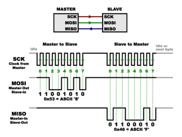
Figure 1.5. SPI master – slave method data transmission
