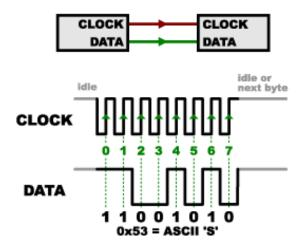
Figure 1.4. SPI interface bits order-using clock and data.
