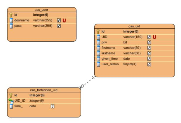
Figure 2.4. Relational scheme of AMCS server side application's database
