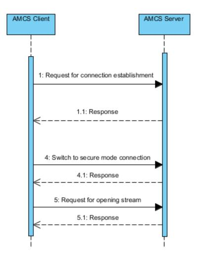
Figure 2.7. AMCS client – server communication principle
