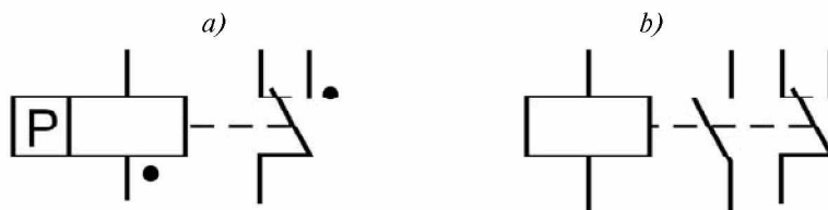
6.3-rasm. Relelarning sxemalarda shartli belgilanishi: elektromagnit (a) va qutbli (b).
