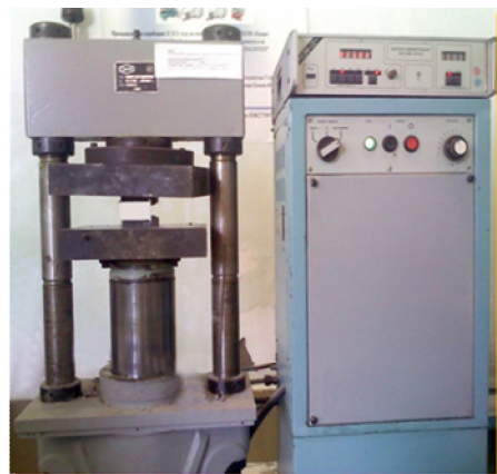
5-ustki tayanch plita, 6-namunani mahkamlaydigan burama moslama, 7-manometr, 8-nasos.
