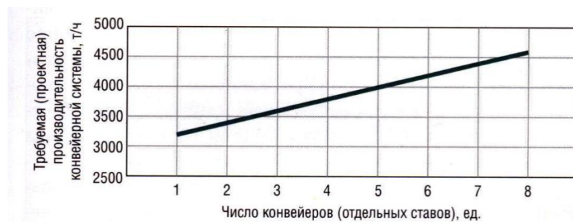
Figure 2.7 Dependence of the design technical performance of the conveyor system on the number of individual stages (included in the conveyor system)
